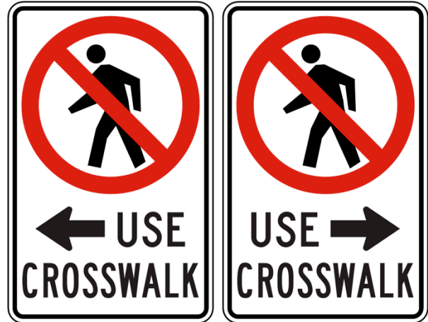
“Use crosswalk” signs to be used to direct pedestrians to crossing. 300 x 450 mm and 600 x 750 mm.
