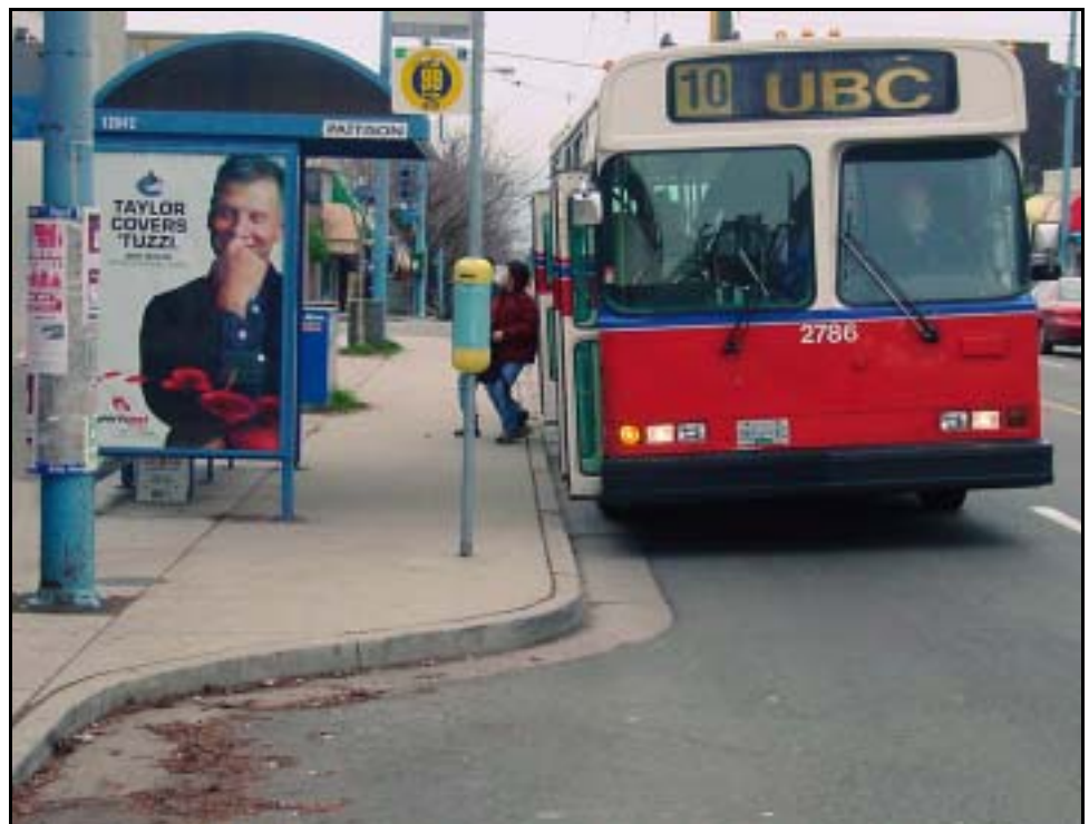
Figure 4.7: Bus Stop with Bus Bulge – Westbound 10 th Avenue at Sasamat Street
