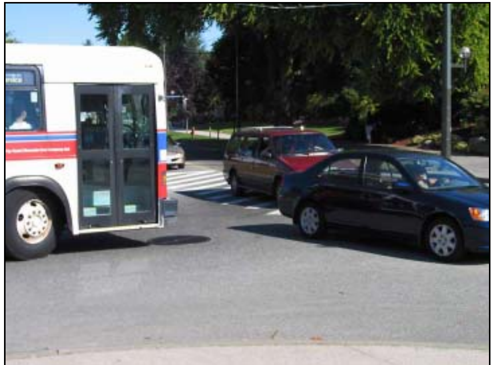
Figure 2.16: Bus Blocked at Bus Loop Exit
